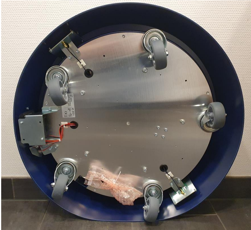
Figure 7: Log & Guard B:safe monitoring trolley on its side for removal and mounting of the surface temperature sensor.
