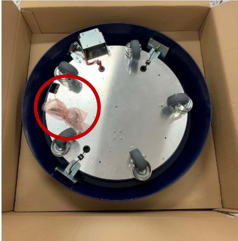
Figure 3: Loose holder with the surface temperature sensor attached to the underside of the monitoring trolley.
