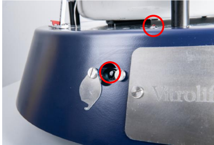
Figure 16: Tare button and LED.
