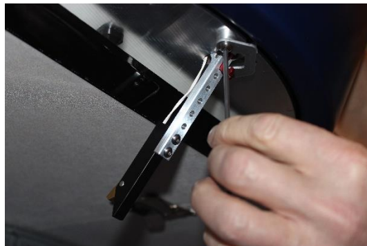
Figure 8: Surface temperature sensor being fixed to the trolley from below.
