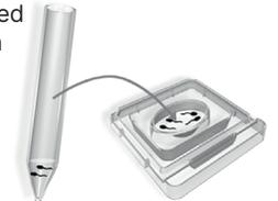
If oil overlay is used, droplets of at least 100 µL volume are recommended. Equilibrate the dishes at
