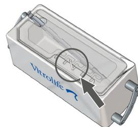
The lowest black mark of the Rapid-Straw must always be submerged in liquid nitrogen.
